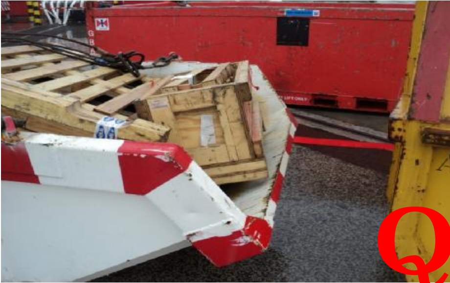
Wooden box loaded on sloping side of open waste skip
