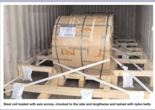
Steel coil loaded with axis across, chocked to the side and lengthwise and lashed with nylon belts
