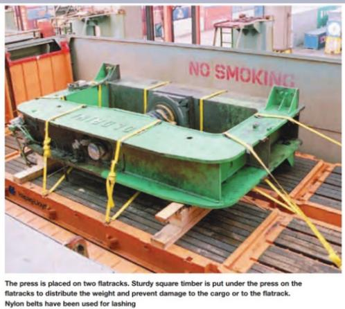
The press is placed on two flatracks. Sturdy square timber is put under the press on the flatracks to distribute the weight and prevent damage to the cargo or to the flatrack. Nylon belts have been used for lashing
